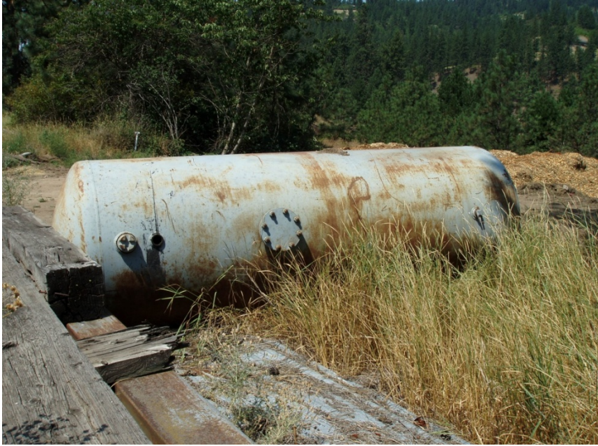
Figure 4, Creosote pressure tank, located offsite on Dale Richardson's property, Orofino-Riverside.
