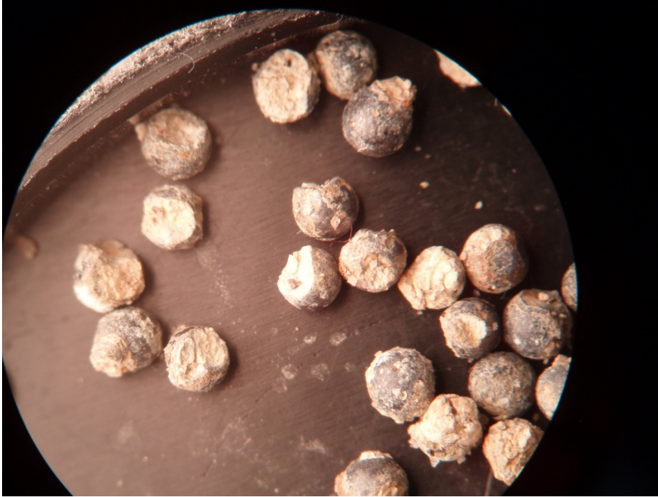
Figure 6. Lead shot collected from riverbank of TU-46 downrange of Orofino Trap House.
