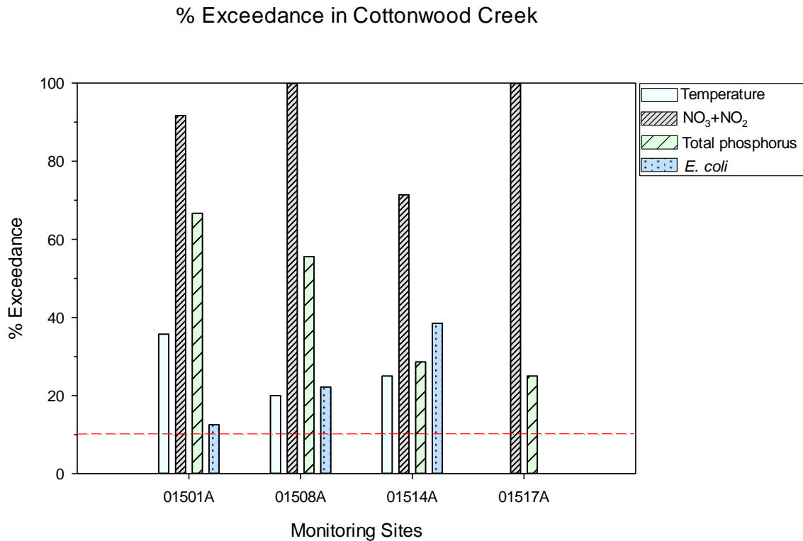
Figure 30. Percent exceedance of instantaneous parameters (temperature, nitrate+nitrite, total phosphorus, and E. coli ). Sites are positioned from mouth to headwaters from left to right respectively. E. coli was calculated by including samples analyzed by both the NPT and BOR.
